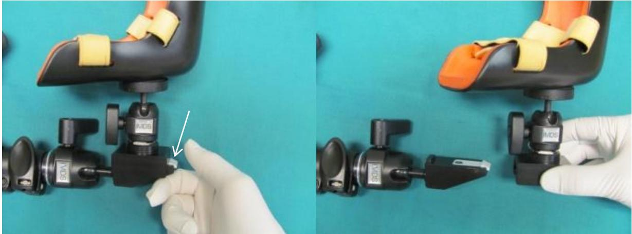
2 Tighten the screw of the quick release adaptor with **2.6Nm** by using a Torque wrench with a Phillips PH2 Bit.
