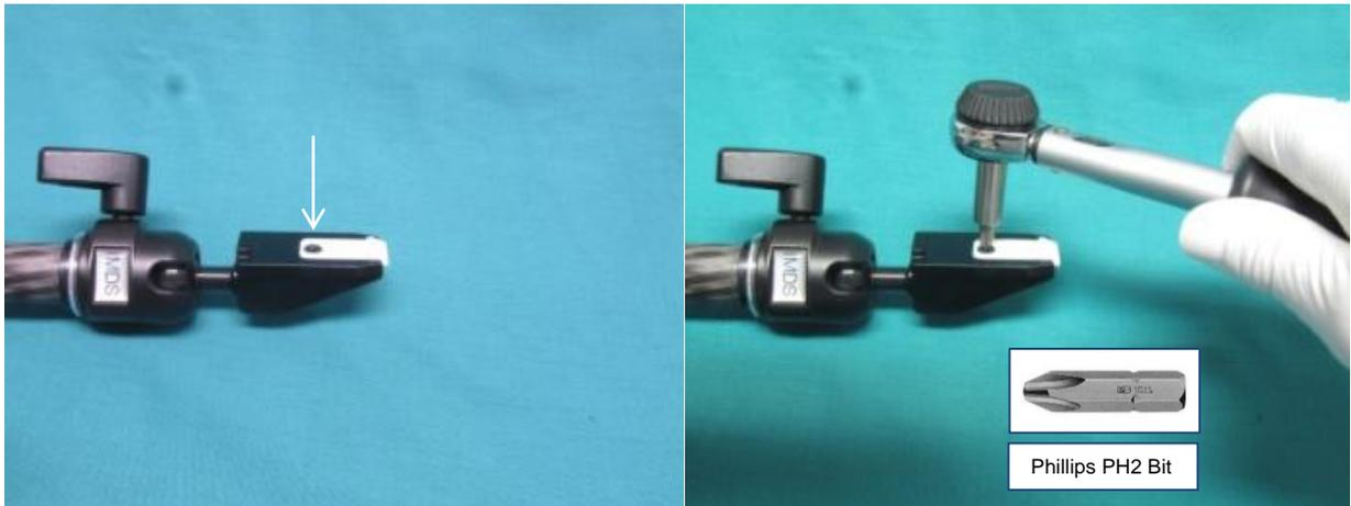
3 Do not remove the bolts of the friction mechanism by completely disassembling them. These bolts consist of 2 parts that can easily be lost. As a consequence the clamp function will not work anymore.
